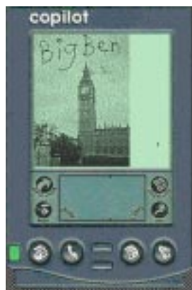
Figure 18: Top Gun MediaBoard allows the PalmPilot to participate in shared-whiteboard sessions, despite its small display and inability to support the Scalable Reliable Multicast protocol on which the original MediaBoard is based.
